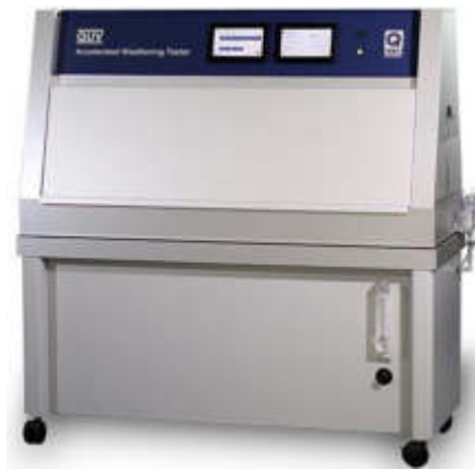
Figure 2 Q-LAB QUV accelerated aging test chamber [9]
