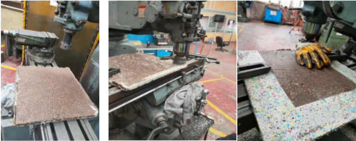
Figure 4: The view of machining of the produced plate
