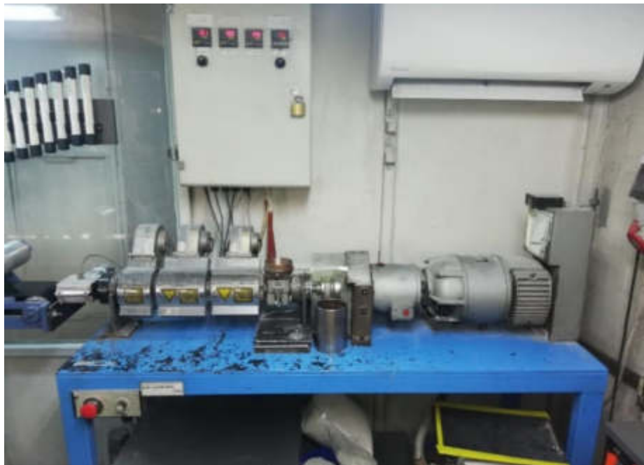
Figure 3: Laboratory type extruder machine
