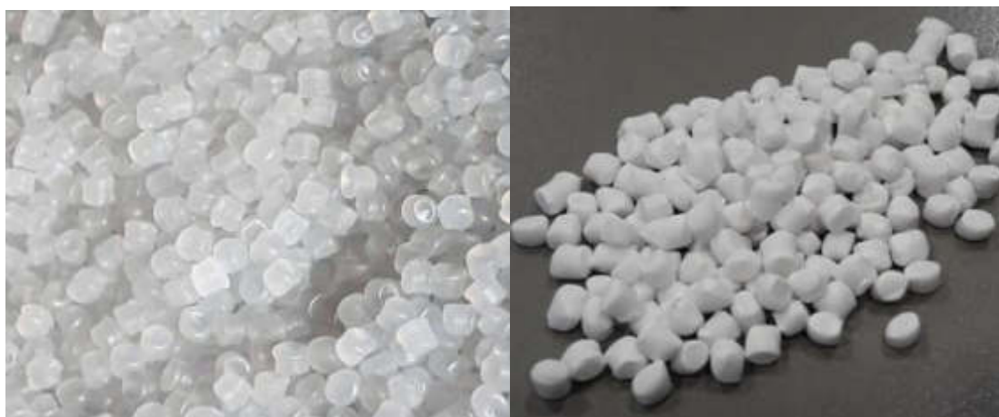
Figure 2 On the left, LDPE SABIC 2200 H0 granules, on the right, filler \text{CaCO}_3 WD-FM 801 [own materials]
